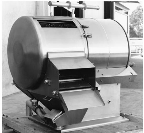
The Brown Model 1100 Citrus Extractor is installed in a citrus processing line to extract the lemons and limes and is configured to accommodate each fruit size. Each size extractor tolerates significant overlap of fruit sizes making efficient use of all the extractors on each processing line.
