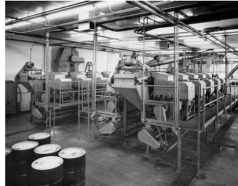
The function of the machine is to shave the peel to remove rag or separate various amounts of albedo (white layer) from the flavedo (colored layer) of the peel. The essential oil is recovered from the flavedo, which contains the oil sacs. The albedo is used for pectin production and other products.
