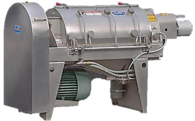
**APPLICATIONS:** The Model 2503 is readily adapted to extracting, finishing, de-watering, and separating with a minimum degradation of solids. Citrus products as well as other diverse materials such as apricots, tomatoes, pears, apples, plums, grapes, and pineapple have the liquids satisfactorily separated from the solids. The Model 2503 provides rigid quality control, easy cleaning and low maintenance.
