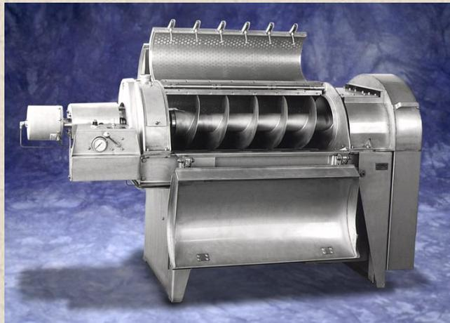
**SMOOTHER OPERATION:** The Model 2503 operates smoothly and efficiently with a minimum of attention. Plugging is eliminated because of the positive conveying action of the screw.
