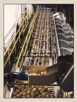
**APPLICATIONS:** The Model 5500 is readily adapted to accurately size and distribute various types of citrus fruit for processing. The volume of fruit to be processed and the types and numbers of extractors to be utilized determines the configuration of the sizer. The configuration of the sizer is the combination of the number of "runs" or sizing lanes and the length of the sizer or number of "bays".
